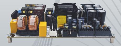
The PS500 is a high efficiency Safety Class 2 switch mode power supply specifically designed to be used in combination with single or dual Nilai500 modules. Its key features are high efficiency over the entire load range, use of audiophile components and interleaved PFC for increased power density and lower conducted EMI.
