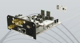
The PreDIGin add-on is designed to complete the Hypex Direct PreAmplifier. PreDIGin is the digital companion for audio enthusiasts seeking the ultimate listening experience. At the heart of the PreDIGin lies cutting-edge technology, including high-quality components such as the AK5574 ADC IC, dual CS43198 DAC ICs operating in mono mode, SRC4392 for superior sample rate conversion, and the ADSP21489 DSP for advanced signal processing capabilities.
