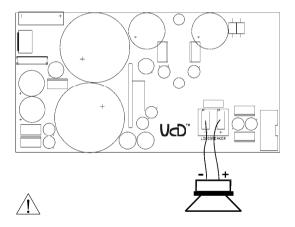
Be sure to disconnect the DS4.0 from the mains before proceeding! Connect the loudspeaker, wired with wire of sufficient cross-section (1.5mm² or 15AWG), to + and - as shown in the picture above. Use 6,3x0,8 FASTON® connectors and crimp them with a suitable crimp tool. Check the voltage selector on the front panel and make sure the voltage is set according the mains voltage used in your country.
