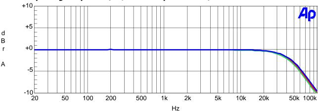
From top to bottom: open circuit,  $8\Omega$ ,  $4\Omega$
